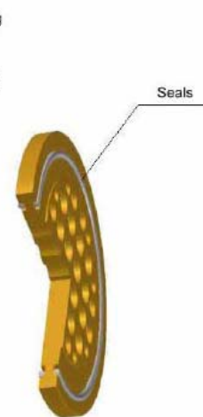
Figure 3 Zanker Board-type Flow Conditioner
